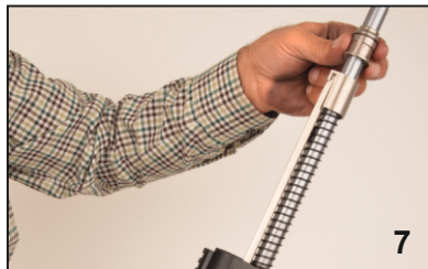
7. Remove the plunger
