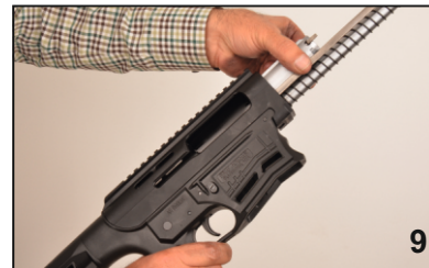
9. Remove the mechanism
