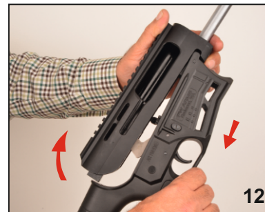
12. Seperate the receiver into two
