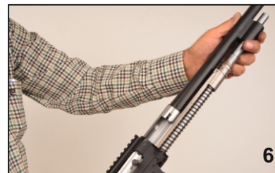
6. Remove the barrel
