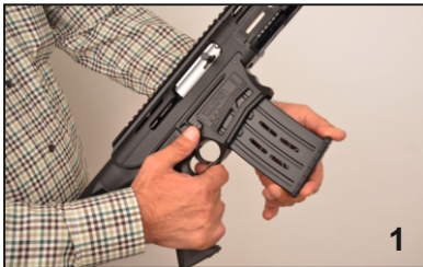
1. Press the latch remove the magazine
