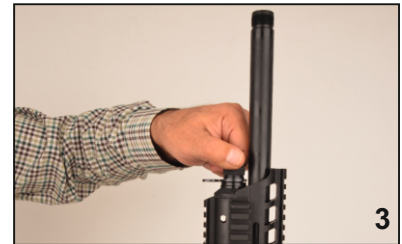
3. Remove the magazine cap
